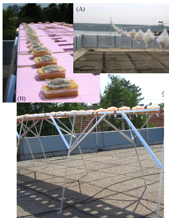
Fig. 1. Experimental setup: (A) dry, and (B) wet moss bags.
